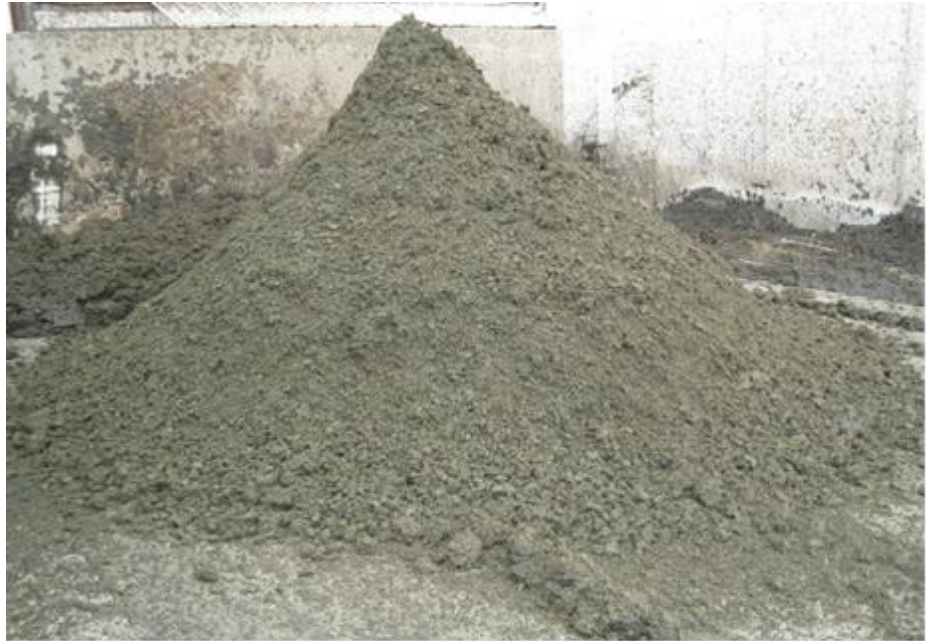
Stacked nutrient fertilizer with 85% of the phosphorous, 50% of the nitrogen, and 20% of the potassium captured.
